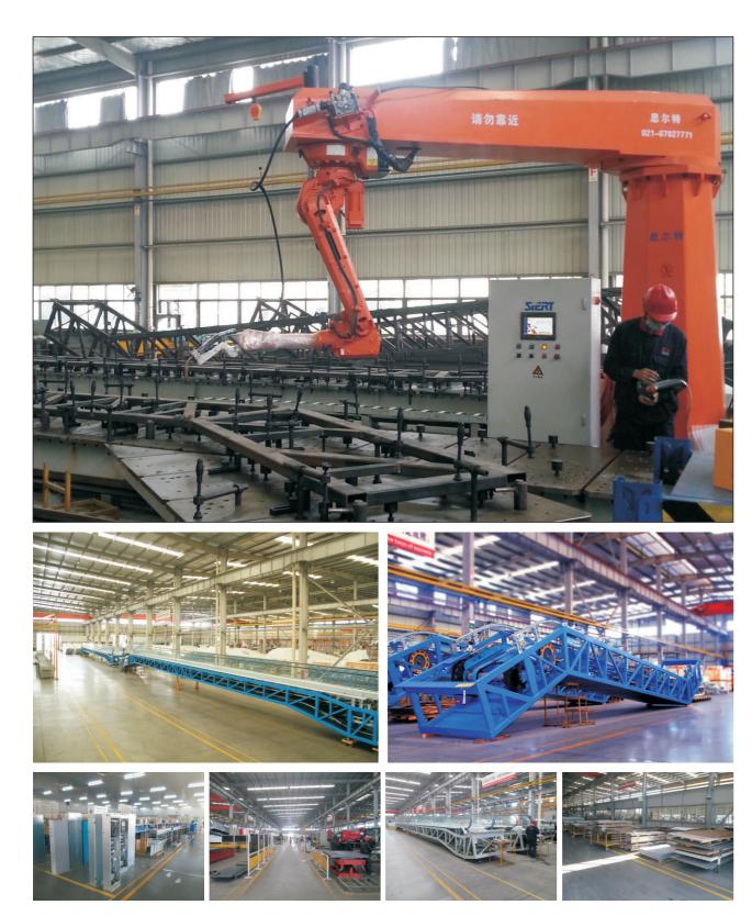
Equipment performance: used for escalators truss welding.
