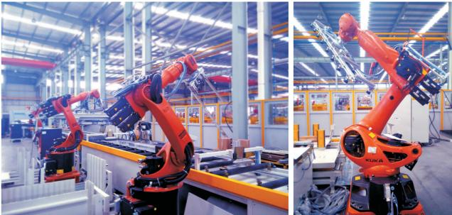
Summary: This highly intelligent and flexible production line no need any treatment for WIP, and complete sheet metal punching, bending, cleaning, gluing, riveting, thus producing sheet metal automatically. Under the premise of not occupying any production flow time, the flexible programming and automatic setting enable the unmanned production become reality which is economic in lean production.
